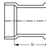
For connection to Cast Iron system. Requires packing and plastic lead. **Warning:** Do not use hot lead or oiled Oakum.
