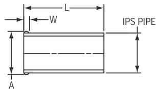
For connection to glass system. Requires use of clamp from glass system manufacturer.
