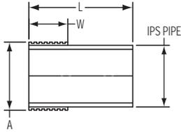
For connection to Duriron system. Requires duriron mechanical joint coupling.
