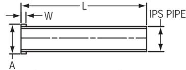
For connection to Duriron system. Requires packing and plastic lead. **Warning:** Do not use hot lead or oiled Oakum.
