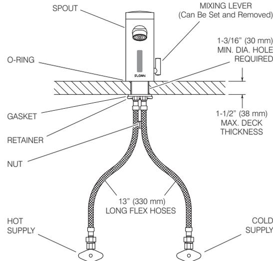
When the EAF faucet is installed on a sink that has three (3) hole punchings, a Trim Plate should be used.
