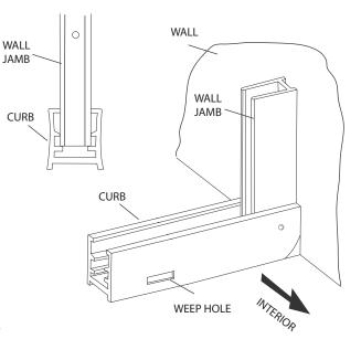
**5** Wipe the shower walls, sill, curb & wall jambs with a clean, dry cloth to remove any dust or debris. Apply a 1/4" bead of silicone along the inside of the pencil lines that were marked in Step #3. Carefully place the curb on the sill, over top the silicone, in the position marked.
