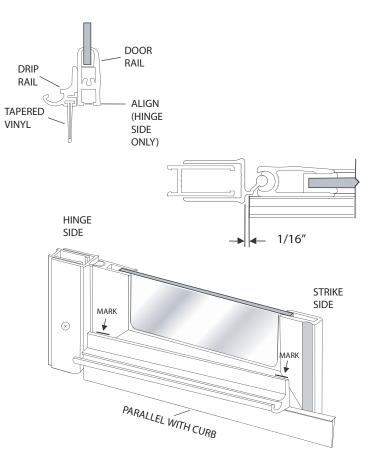
**12** Hold the drip rail in place and adjust the drip vinyl by sliding it left or right until there is a 1/16" gap between the bottom of the vinyl and the top of the snap-in-filler. Trim the vinyl flush with the hinge side of the rail and 3/8" longer on the strike side. Notch the top of the drip vinyl. (see illustration)
