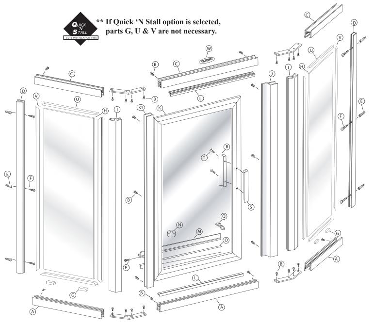
**1** The Framed Continuous Hinge Shower door panel is completely reversible and may be installed hinge right or hinge left. For maximum waterproofing, the door should hinge off of the panel opposite the shower head wall. (see illustration) Careful as to not follow the illustrations exactly.
