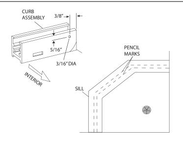
4 Place one wall jamb [D] into the curb against the wall. Using a level, plumb the wall jamb and mark the hole locations on the wall with a pencil. Repeat this step for the other wall jamb. Remove all parts and drill the holes. **TIP:** Tape can be used to temporarily hold the curb in place.
