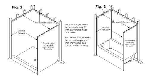
IF A BEDDING MATERIAL IS USED UNDER A UNIT; CEMENT SLURRY, THIN MORTAR MIX, PLASTER OF PARIS, OR A COMPARABLE FLOOR FILLING COMPOUND THAT IS NOT WATER SOLUBLE ARE PROPER BEDDING COMPOUNDS. WATER SOLUBLE MATERIALS, FOAM AND OTHER EXPANDING MATERIALS ARE NEVER TO BE USED AS A BEDDING COMPOUND.
