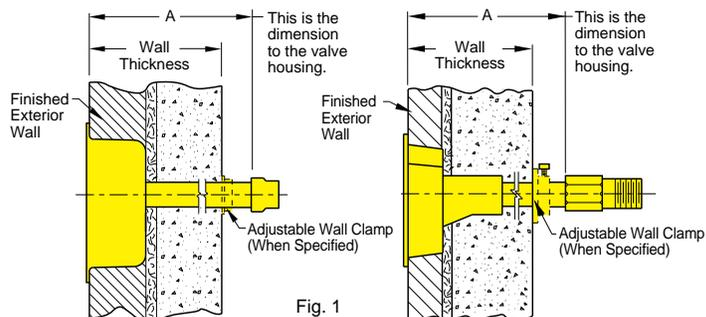
**NOTE:** When ordering, specify Figure Number and "A" dimension. "A" should always be greater than wall thickness for non-freeze installations. When a wall clamp is specified, add 1/4" to the wall thickness to arrive at a minimum required "A." The "A" specified should be the next larger, even number; such as 6", 8", 10", etc. Wall hydrants are furnished in lengths of 2" increments.
