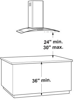
The vent hood must be installed 24" min. and 30" max. above the cooking surface depending on the ceiling height.
