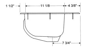
Dimensions shown are for reference. Actual dimensions may vary slightly and should be checked prior to installation.
