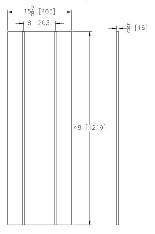
Engineering Specification: Zurn non-structural Thermal Track™ straight panel. This 5/8" thick panel is comprised of Medium Density Fiberboard (MDF) with a highly conductive aluminum layer bonded to the surface. The straight panel is 16" x 48" and contains two parallel grooves milled at 8" on center. The grooves accept 3/8" PEX Barrier and Performa® tubing. Each panel weights approximately 44-50 lbs. per cubic foot (13.3 lbs. per panel).
