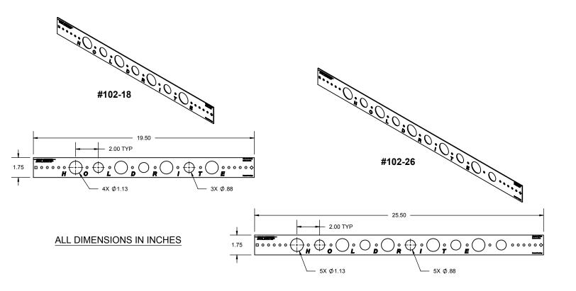
The HOLDRITE #102-18 and #102-26 are Copper-Bonded™ steel brackets with holes to support 3/4" and 1" copper tubing. Used to support stub-outs for hot water tanks, urinals and other fixtures. When soldering, heat the pipe, not the bracket.
