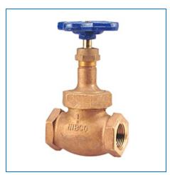
**Specifications UPC** Code 039923627681 Type Globe Valve **Valve Size** 1 1/4 T -- Female NPT Thread (FIPT) **Connection Type** Material **Bronze** Standard Handwheel **Valve Operator** T235Y 1 1/4THD 150# GLOBE W/PTFE SEAT **Description** eClass Classification Bronze Globe Valves **Turns/Operation** Multi-Turn Weight 5.757 lb
