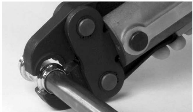
**Figure 10 – Opening the Jaw set and Placing Around Fitting**
