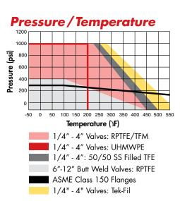
**NOTE:** Series 8000 Carbon steel valves are limited to -20°F.
