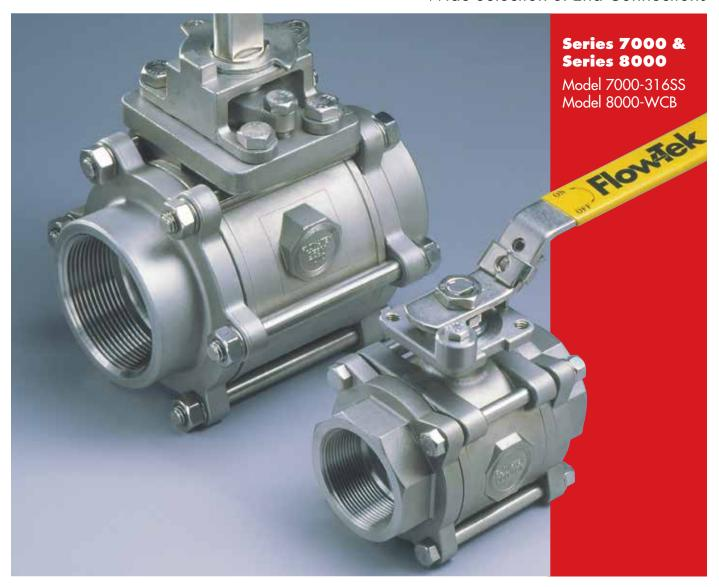
Flow-Tek's Series 7000 & 8000 ball valves offer the highest flexibility in selection of end connections, seat materials and 3 piece design. To meet customer demands for a valve with the widest possible range of applications, these valves can be fitted with control or tri-ported balls (for full cavity drainage), as well as cavity fillers for special service requirements.
