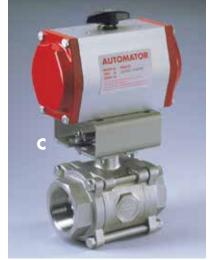
Secure Mount (C) The integrally cast top flange ensures positive actuator mounting. Secure Mount eliminates unwanted actuator movement during high cycle or continuous duty applications. Actuation equipment can be easily and safely removed while the valve is under full line pressure. Designed to ISO 5211 bolting pattern standards.
