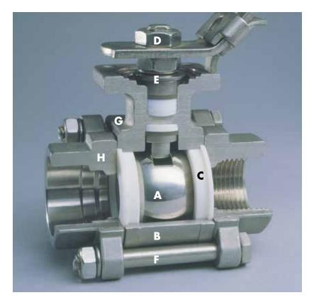
**Ball (A)** Flow-Tek balls are precision machined and mirror finished for bubble-tight shut off with less operating torque. Ball edges have machined curvatures to reduce seat wear and provide a high cycle life.
