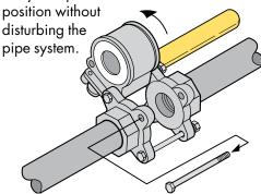
Out of Line Servicing For complete removal of valve from the line, remove the upper two bolts that go through the body hinges, loosen the lower two while keeping them in line, then lift the valve body out of the pipeline. The remaining two bolts keep the pipeline system in place and maintain alignment. The removed body
