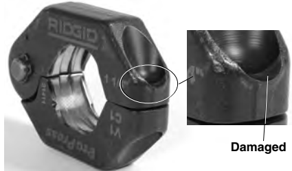
Figure 11 – Damaged Ring Pocket
