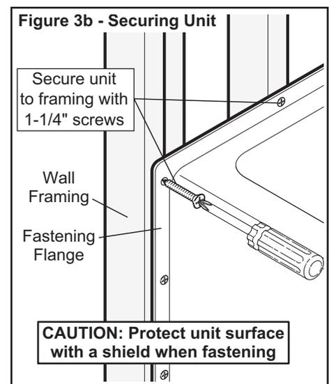
The unit must also be positioned square in the alcove framework. The use of shim or filler material behind the fastening flange at each framing member may be required to maintain the unit in the proper position.
