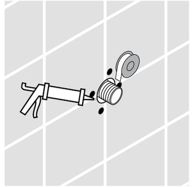
Install the anchors. Seal the wall around the anchors with waterproof sealant.
