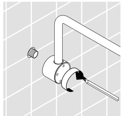
Wrap the threads on the nipple with Teflon thread tape.
