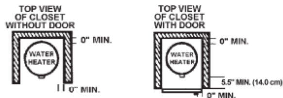
Figure 6. Wall Clearances for Water Heater Installed in a Closet.
