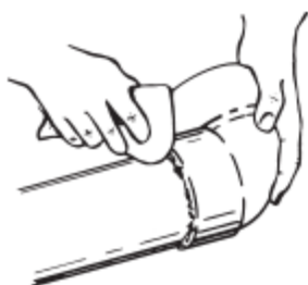
Figure 23. Step G, Cleaning Up the Joint
