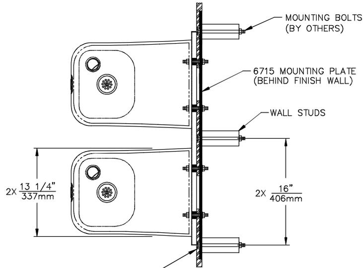
FINISH WALL OVER MOUNTING PLATE AND BEHIND BACKPANEL. BE CAREFUL THAT FINISHED WALL EXTENDS WITHIN THE HAWS BACKPANEL.
