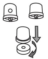
To install, simply plug-in and twist clockwise.
