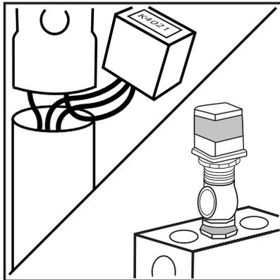
1. **Do not face the photocell into the midday sun.** If installed on the south side of a building, face east or west or point the photocontrol down toward the ground. The best direction to face the photocontrol is north.
