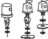
All mount in any approved outdoor FS box or in a fixture with 11/16" or 3/4" diameter hole.
