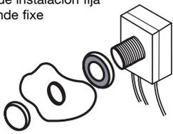
Mount in approved FS box or fixture with 11/16" or 3/4" diameter hole.
