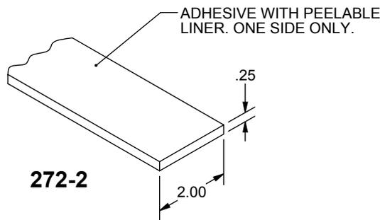
**Felt #272-2 HOLDRITE® Isolating felt for use in eliminating dissimilar metal contact and providing sound and vibration isolation. One side is self-adhesive. Available in 25' roll.**
