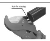
Reaming & deburring can be done using the hole on the blade. This is only for outside edge of pipe.
