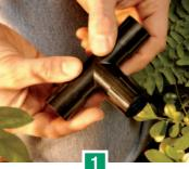
Select an Easy Fit Compression Select the Easy Fit Fitting—either a coupling, an elbow or a tee.
