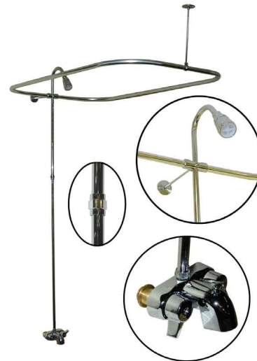
#687 61-1/4" Height CP Bathcock Diverter w/3-3/8" Center 27" x 42" Aluminum Curtain Ring 10" Wall Support & 36" Ceiling Support Set screws allow supports to be cut to the desired length. Only the flange end is threaded
