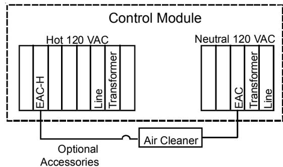
If it is necessary for the installer to supply additional line voltage wiring to the inside of the furnace, the wiring must conform to all local codes, and have a minimum temperature rating of 105°C. All line voltage wire splices must be made inside the furnace junction box.
