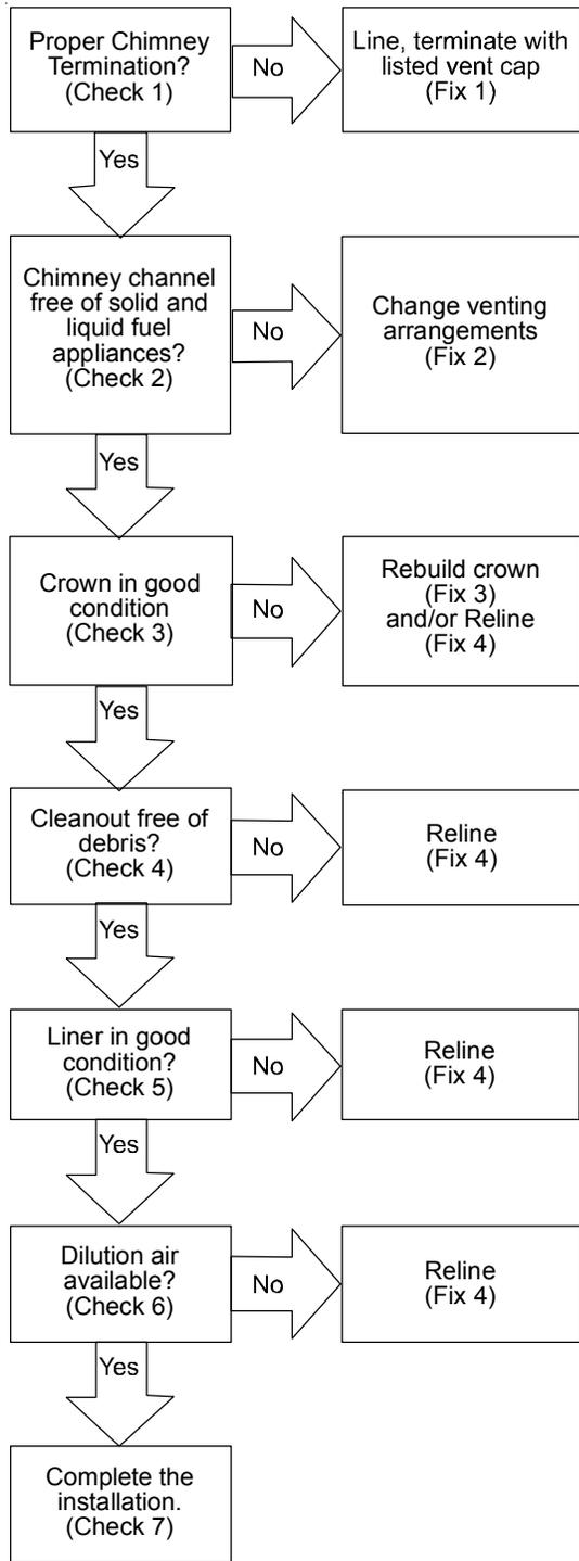
If the chimney does not meet these termination requirements, but all other requirements in the checklist can be met, it may be possible for a mason to extend the chimney. If this will not be practical, see Fix 1.
