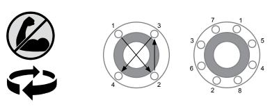
Do not over tighten. Flange bolts should be gradually tightened across Use correct torque figures. diameters to ensure even load and alignment.
