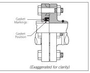
4. **INSTALL GASKET:** Install the gasket onto the pipe end. Make sure the gasket is positioned properly, as shown above. **NOTE:** The lettering on the outside of the gasket must face the gasket seating area of the Style 441 Vic-Flange Adapter.
