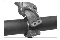
**6. INSTALL HOUSINGS:** Install the housings over the gasket. **NOTE:** The housings are clearly marked "Grooved End" and "Plain End." Make sure the housings' keys engage the groove and that the plain end aligns with the pipe marks. Make sure the gasket remains in position and that the tongue and recess features of the housings mate properly (tongue-to-recess).
