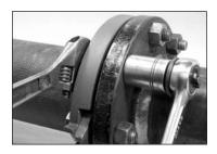
**8. TIGHTEN NUTS:** Tighten the nuts evenly, as with a regular flange assembly. Continue tightening until the flange faces come into metal-tometal contact or the bolts reach the standard flange-joint torque requirement.
