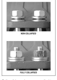
Collapsible washers are supplied to ensure proper penetration of the teeth into the pipe. The collapsible washer is designed to collapse under a predetermined load, which provides the required compression for full joint performance. The collapsible washer provides a visual check for proper tightening of nuts.
