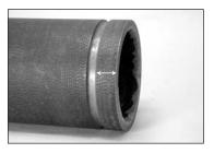
1. CHECK PIPE ENDS: The outside surface of the pipe, between the groove and the pipe end, must be smooth and free from deep pits and swells to provide a leak-tight seal for the gasket. All rust, loose scale, oil, grease, dirt, and cutting particles must be removed. Peened surfaces may require rework to provide a leak-tight seal for the gasket (refer to ANSI/AWWA C-606 or CSA B242).
