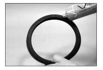
2. CHECK GASKET AND LUBRICATE: Check the gasket to make sure it is suitable for the intended service. Apply a thin coat of Victaulic Lubricant or silicone lubricant to the gasket lips and exterior. NOTE: This gasket is designed to provide the primary seal. Refer to page 43 for special applications.
