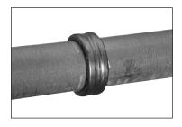
**4. INSTALL GASKET:** Install the gasket onto the pipe until the pipe end contacts the center leg of the gasket. Insert the other pipe into the gasket until the pipe end contacts the center leg of the gasket.
