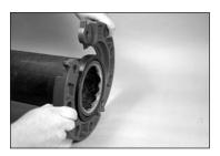
**4. INSTALL VIC-FLANGE ADAPTER:** Open the hinged Vic-Flange Adapter fully, and install the flange over the gasket. Make sure the key section of the flange adapter engages the pipe groove properly.
