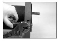
**5.** While squeezing the closure lugs together, insert a standard flange bolt through each of the two mating holes in the Vic-Flange Adapter; this will maintain the position of the flange in the groove.
