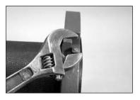
Closure lugs are provided for ease of installation. If necessary, use an adjustable wrench to align the mating holes.
