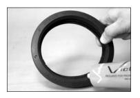
2. CHECK GASKET AND LUBRICATE: Check the gasket to make sure it is suitable for the intended service. Apply a thin coat of Victaulic
