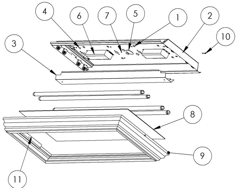
NOTE: It is possible to remove the lamps and diffuser without removing the frame from the fixture.
