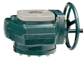
M31 - Variable torque advantage output for reduced input force, cast iron housing, bronze and steel internals, roller bearings, direct mount limit switch capability, visual indication, epoxy coated.
