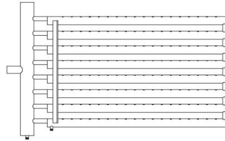
To prevent condensation on in-duct objects, such as dampeners, coils, filters or turning vanes, it is very important that the dissipation distance be shorter than the distance from the humidifier to the in-duct object. The following recommendations should be used when designing a multiple injection tube system:
