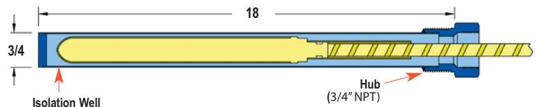
**For deeper & variable insertion depths into tanks or vats; up to 18" deep.** The extended length Isolation Well isolates the copper sensing bulb from the liquid and allows the copper sensing bulb insertion depth to be adjusted to a depth of up to 18". They are available in either Brass or 316L Stainless Steel. Isolation Well remains in place which allows the removal of the sensing bulb without having to drain the tank.
