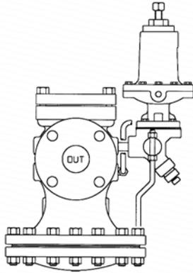
Shown with **PP** Pressure control Pilot. Spring-loaded pressure pilots are the most typical method of controlling downstream pressure in Steam Systems. Adjustment screw on top of pilot controls downstream steam pressure.
