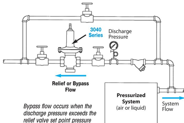
Bypass flow occurs when the discharge pressure exceeds the relief valve set point pressure
