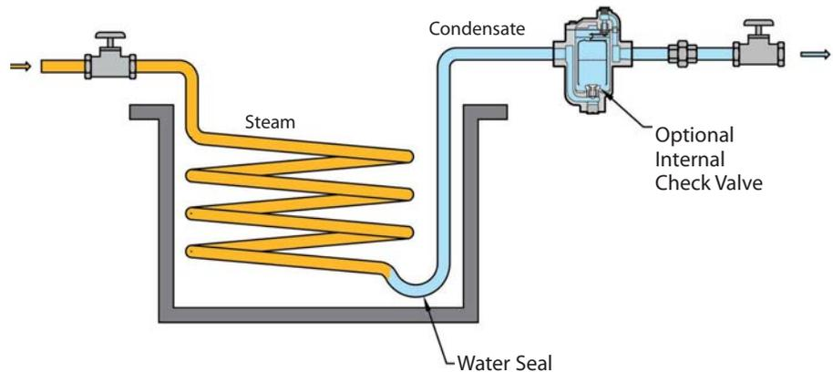
**Steam Trap Discharging into Elevated Condensate Return Line**
