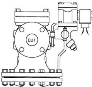
Shown with **PS ON-OFF**(solenoid Pilot) control pilot: The **PS ON-OFF** (solenoid) Pilot allows for the HD valve to be opened and closed using an electrical switch to activate a small solenoid valve. The **PS** Pilot can be used for system automation or as a safety shut down device. The ON-OFF pilot is most often used in conjunction with a Pressure or Temperature control pilot.
