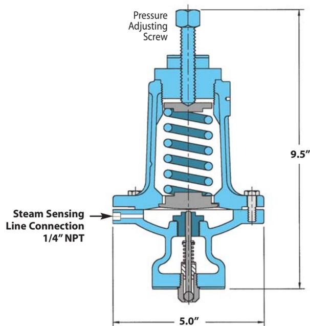
**Back Pressure Regulating with PBP Back-Pressure Pilot**
