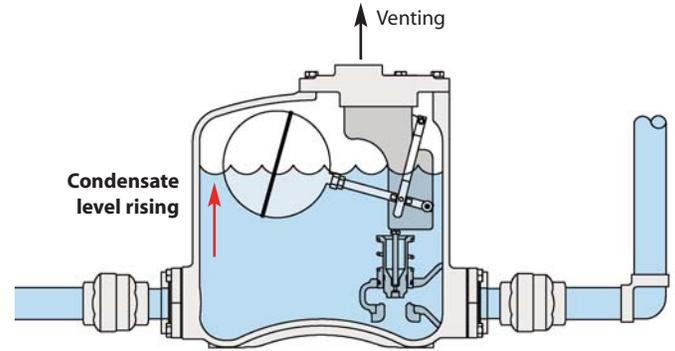
**2 PUMP TANK FILLS:** Inlet steam pressure falls below back pressure. Steam can no longer push the condensate through the Steam Trap.
