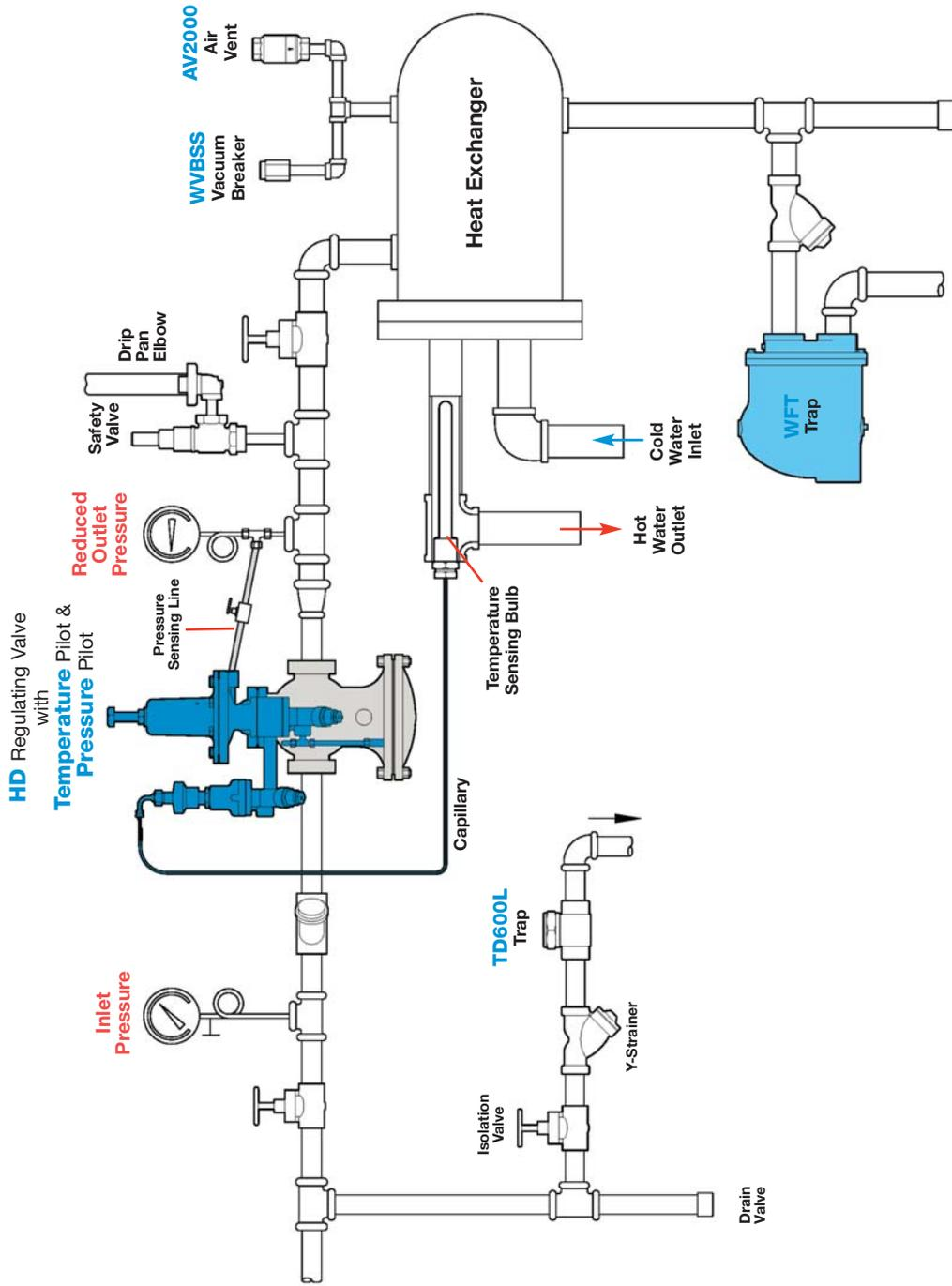
Temperature Control of a Heat Exchanger with Pressure Limiting
