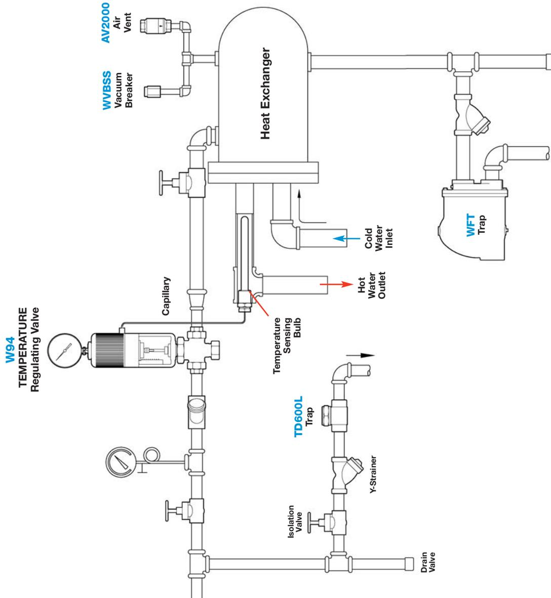
Semi-Instantaneous Hot Water Heater with W94 Temperature Regulator
