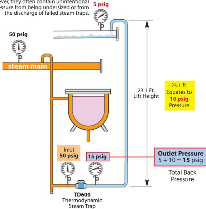
Steam Pressure “pushes” the condensate up through an Elevated return line (15 PSIG)
