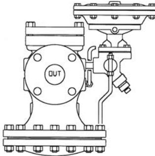
Shown with Air-loaded pressure control pilot. Air-loaded pressure pilots are used to reduce and control pressure in steam systems. They are used as an alternative to the more common spring-loaded pilot. The **PA** Air-loaded pressure pilot allows for remote adjustment of the valve using a small air regulator to alter the air pressure to the top of the pilot.
