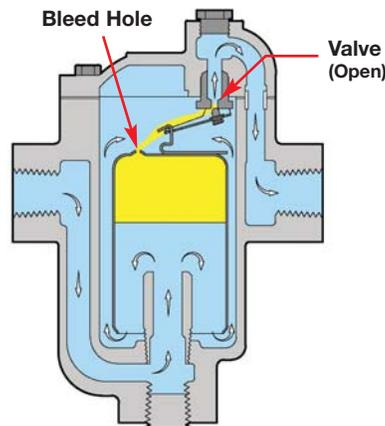
**A)** With condensate completely filling the trap, the bucket is in the down position with the valve open, allowing condensate to be discharged.
