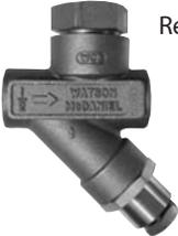
Replacement Capsule Feature | <b>In-line Repairable</b><br>Seat & body are non-integral. Replacement capsule allows for complete repair without removing trap body from piping system. Can be welded in-line. | Alloy Steel         | Drip & Tracing Applications<br><b>30 to 600 psig</b>                                                        |
