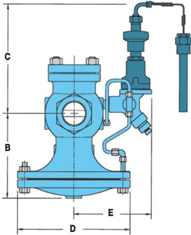
HD Valve with Temperature & Pressure Pilot
