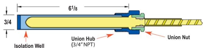
The Isolation Well, which isolates the copper sensing bulb from the process fluid, is available in either Brass or 316L Stainless Steel. Sensing bulb can be removed by unscrewing union nut. Union Hub & Isolation Well remain in place which allows the removal of the sensing bulb without having to drain the tank. Stainless Steel Isolation Wells are used to protect the copper sensing bulb from corrosive fluids. Brass wells have better heat transfer.
