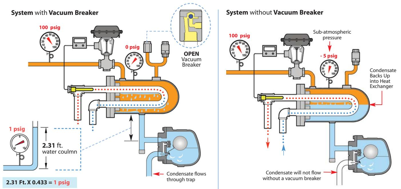
The HX can be properly drained using a steam trap as long as there is no BACK PRESSURE in the condensate return line. If there is back pressure in the condensate return line, a Pumping Trap must be used.
