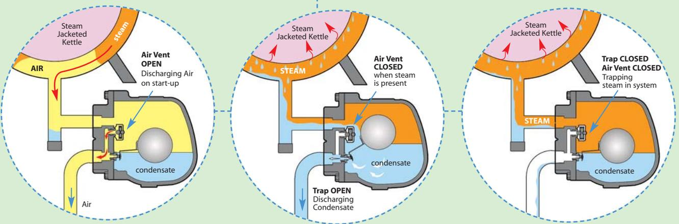
**Process Applications** refer to **removing condensate and air from the actual process** where steam is being used. This process could be a heat exchanger making hot water, or a radiator heating a room, or anything else that requires the use of steam. Traps used for process applications require larger condensate handling capability than steam traps used for drip applications and also need to be able to discharge large amounts of air.
