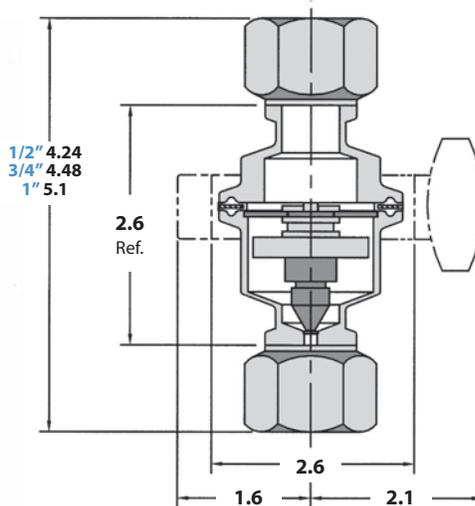
Tube-weld Connection: TW x TW
