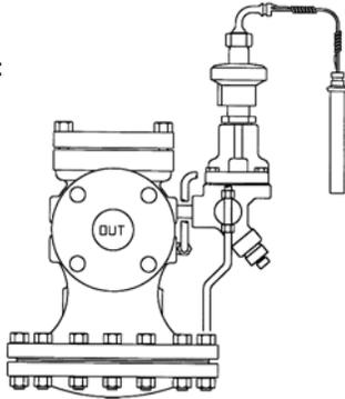
Shown with Temperature control Pilot: The **PT** Temperature Pilot will control the flow of steam flowing through the HD valve based on the temperature of the sensing bulb. The liquid-filled sensing Bulb is available in standard 8 ft and 15 ft capillary lengths. Other lengths available.
