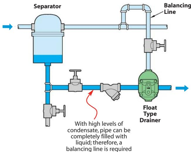
When large loads of condensate are required to be discharged, make sure a properly sized liquid drain trap is used. On large load applications, a balancing line is required, because non-condensable gases can be easily trapped in the drain trap due to fluctuating condensate levels.
