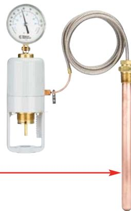
**Model W94 Actuator** is equipped with an integral dial thermometer to indicate sensing bulb temperature. The W94 displays the temperature at the sensing bulb. This allows for easy adjustment of the temperature set-point, as well as continuous monitoring of the application, without the installation of an additional thermometer.
