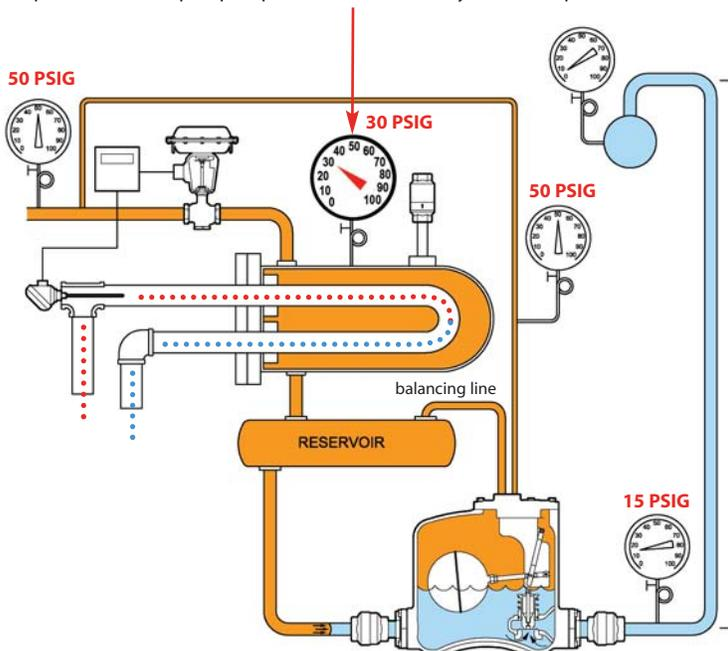
**Vent Outlet:** Open position, allowing pressure in the pump tank to equal pressure in the heat exchanger, allowing condensate to freely enter Pump-Trap by gravity, even under vacuum.
