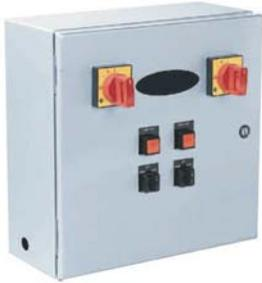
For **Simplex** units, the control panel would include a single motor starter with a single HOA (HAND-OFF-AUTOMATIC) selector switch to turn the pump on manually to verify functionality; or, to set in automatic mode along with a single Motor Circuit Protector switch to shut power off to the pump.
