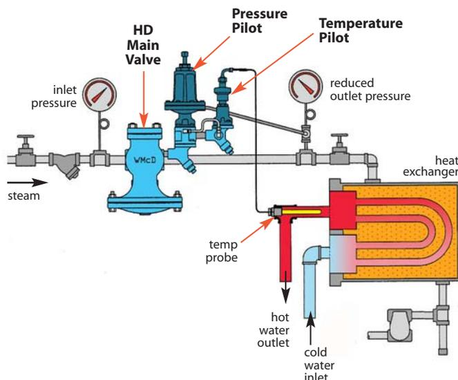
Temperature Regulating with PT Temperature Pilot
