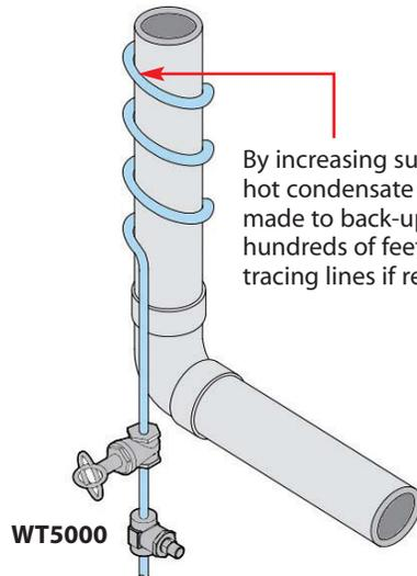
By increasing subcool, hot condensate can be made to back-up into hundreds of feet into tracing lines if required.
