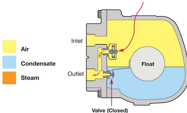
**A)** When cold air enters the trap during start-up, the thermostatic air vent is open, allowing the discharge of large quantities of air from the system.
