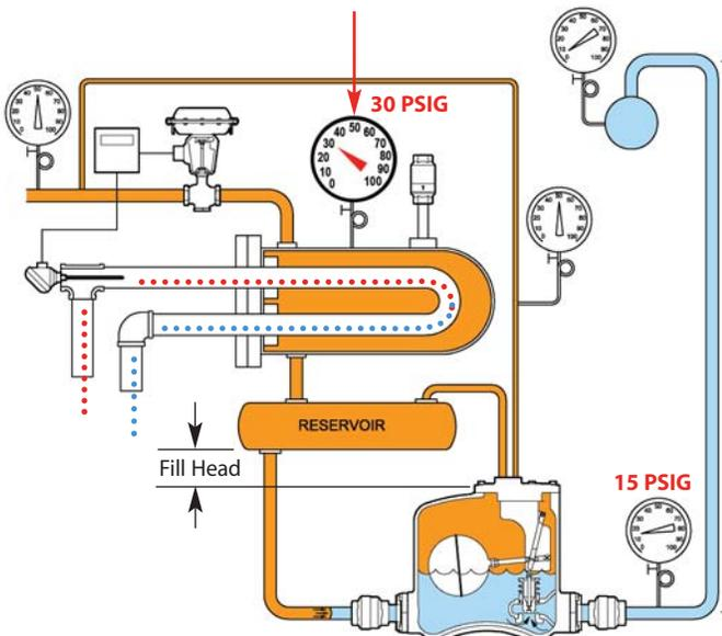
$$\begin{aligned} \Delta P \text{ Trap} &= 30 \text{ psig} - 15 \text{ psig} \\ &= 15 \text{ psi} \end{aligned}$$
