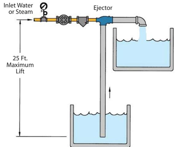
It is always desirable to keep the Ejector as close to the actual liquid being pumped as possible. The maximum height the liquid can be pumped depends upon the pressure of the "motive" liquid or steam available. Please refer to the capacity graphs for maximum flow rates and maximum achievable heads.
