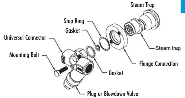
UT450 Trap Module may be mounted in any orientation
