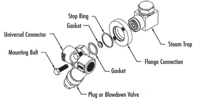
UTD450/UTD600 Trap Module should be oriented with cap facing Upwards, As shown.
