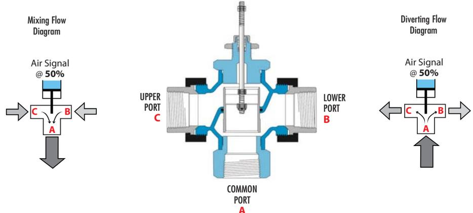
**CAUTION:** 3-Way Valves are not designed for use in steam applications. To properly control the mixing of two flows, inlet pressures at ports B and C should be as equal as possible.
