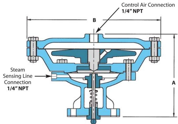
Pressure Control with PA Air-Loaded Pressure Pilot
