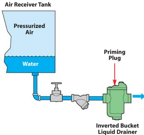
In an application where an Inverted Bucket Liquid Drainer is used, a balancing line may not be required. This style of drainer has a small internal bleed hole on the bucket float which allows a small amount of air to be vented. For the Inverted Bucket Liquid Drain Trap to operate, it must be primed with liquid prior to operation.
