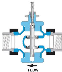
**Normally Closed Valves** are used for **COOLING**, so the valve stem opens (**in-to-open**) as the control signal (temperature) increases.
