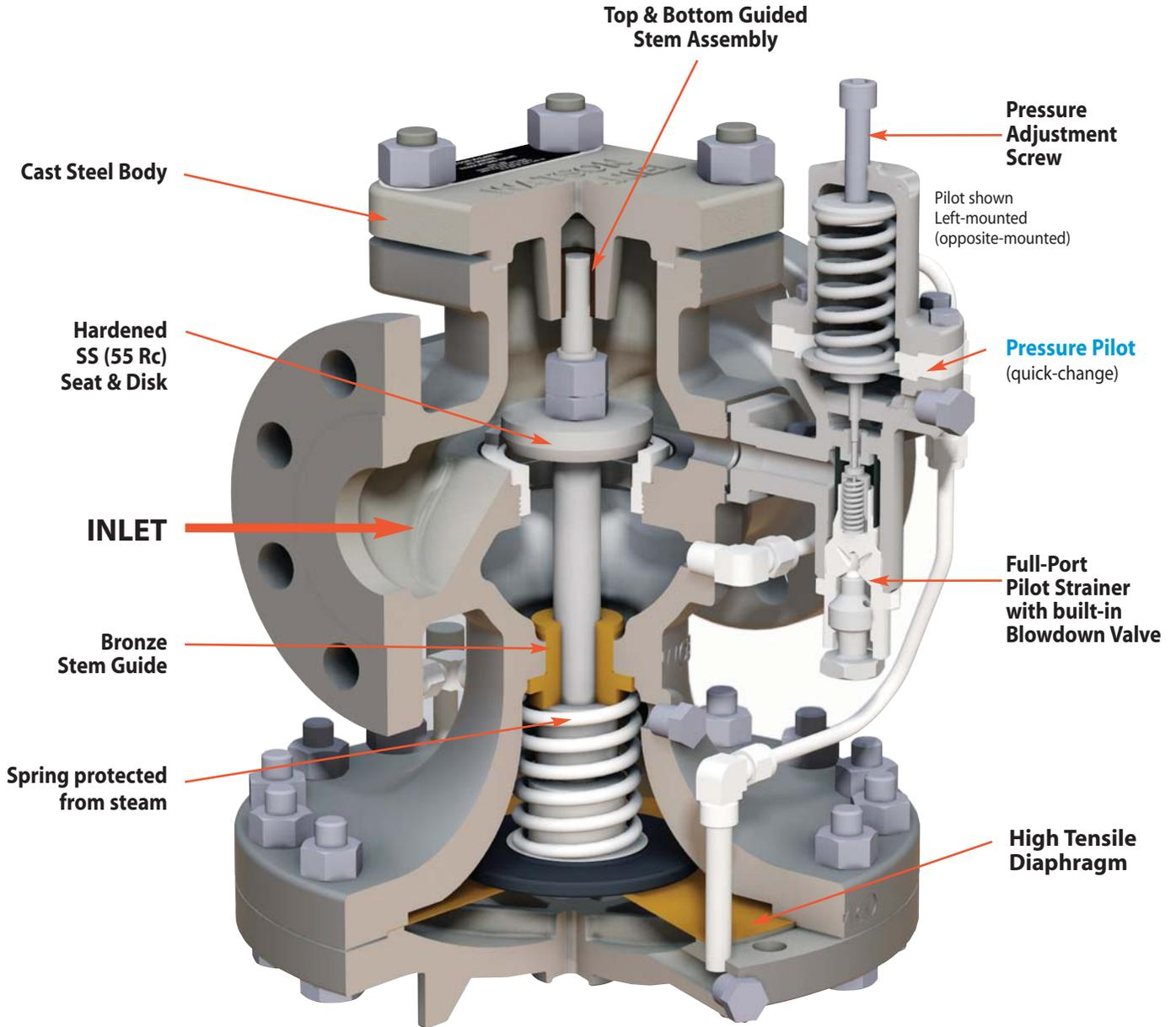
Pressure Regulator shown with Left-mounted Pilot (right-mounted is standard)
