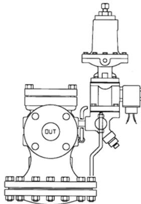
The **PP** Pressure Pilot will maintain the desired downstream set pressure as long as the **PS ON-OFF** (solenoid) Pilot is in the ON position. Available in either Normally-ON or Normally-OFF configuration; an electrical signal turns valve OFF or ON.
