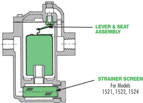
**Lever Seat Assembly with Cover Gasket**
