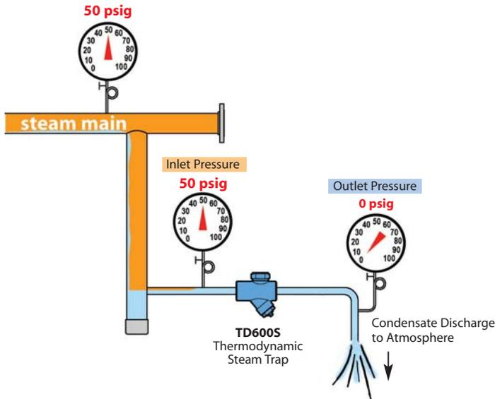
Steam Pressure "pushes" the condensate through the steam trap allowing it to discharge out of the system (0 PSIG)
