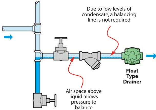
Typically, most air line applications have a low level of condensate to discharge, and the piping does not become flooded with condensate. In this type of application a Float Type Liquid Drainer can be used without the need of a balancing line. Due to the low level of liquid being drained, an air space exists above the liquid in the pipe which balances the pressure allowing liquid to flow freely.
