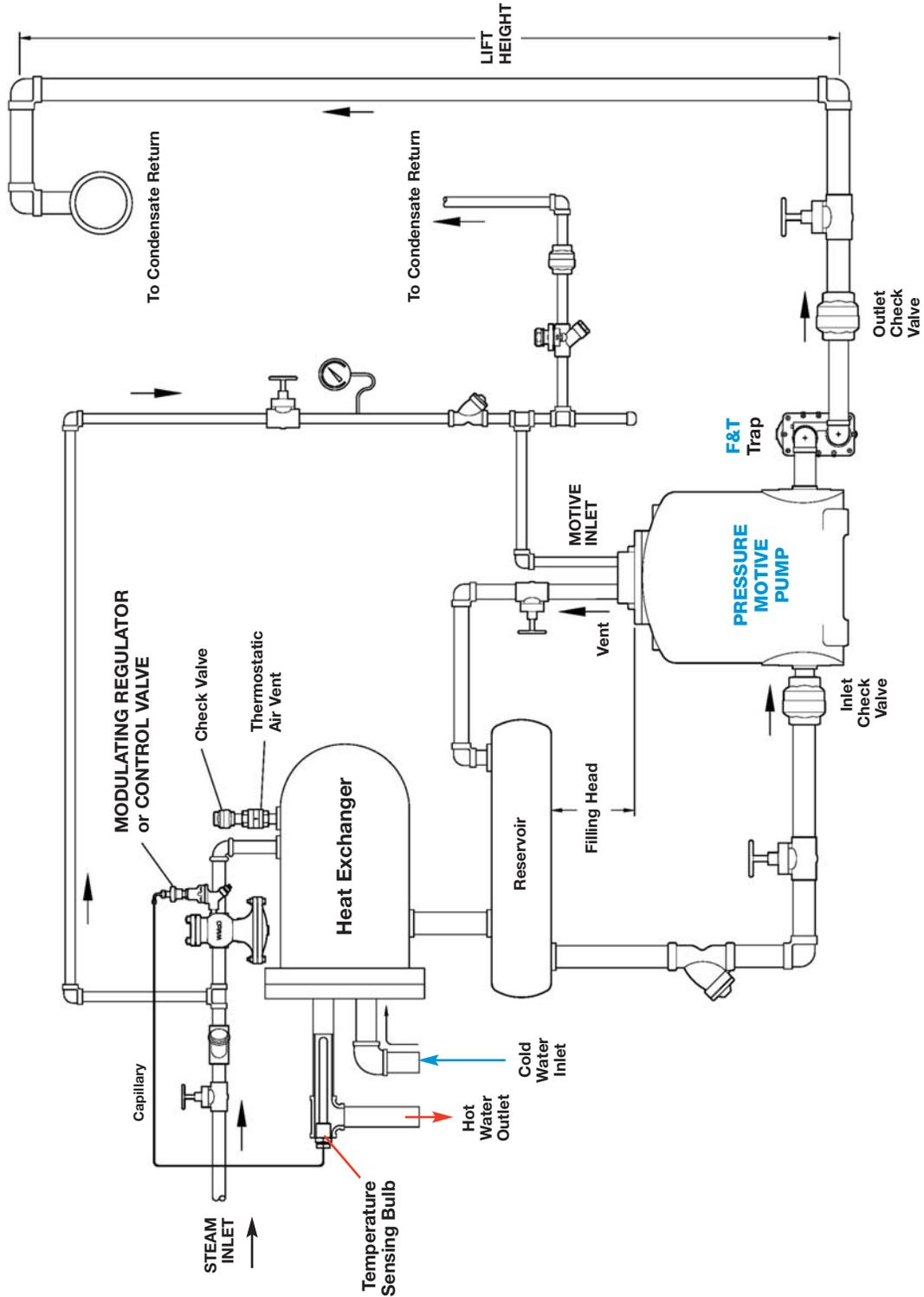
Drainage of a Single Source of Condensate for a Closed Loop System
