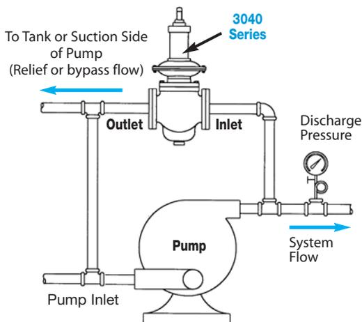
A Relief Valve allows water to recirculate through the pump even when the discharge valve on the pump is completely closed. As a rule, a minimum of 20% of the pump capacity must recirculate to prevent overheating of the pumped liquid.
