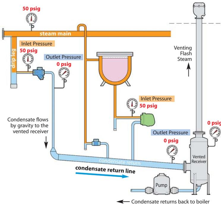
Steam Pressure "pushes" the condensate through the steam trap allowing it to discharge into gravity return line (0 PSIG)
