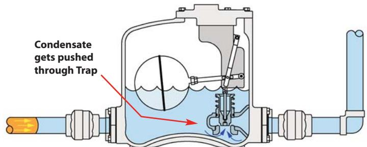
**1 TRAPPING Mode:** Inlet steam pressure is higher than back pressure. Steam pushes condensate through Pump-Trap.
