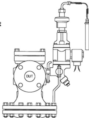
The **PT** Temperature Pilot will maintain the proper flow of steam through the main valve to keep the process it's controlling at the proper temperature as long as the **PS ON-OFF** (solenoid) Pilot is in the ON position. Available in either Normally-ON or Normally-OFF configuration; an electrical signal turns valve OFF or ON.
