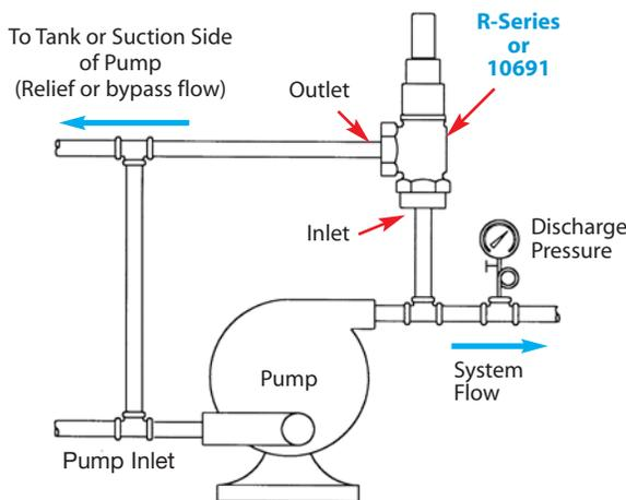
A Relief Valve allows water to recirculate through the pump even when the discharge valve on the pump is completely closed. As a rule, a minimum of 20% of the pump capacity must recirculate to prevent overheating of the pumped liquid.
