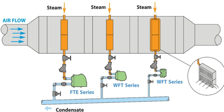
**Multi-Bank Air Heating Coils / Air Handling Unit (AHU)**
