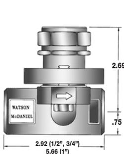
UTD450 Trap Module with UC450 Connector
