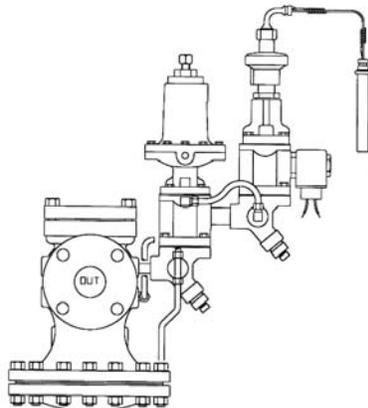
The **PT** Temperature Pilot will maintain the proper flow of steam through the main valve to keep the process it's controlling at the proper temperature as long as the **PS ON-OFF** (solenoid) Pilot is in the ON position. The **PP** Pressure Pilot will **LIMIT** the downstream pressure to a maximum value.
