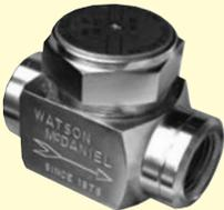
No Strainer                   | The one piece body-seat design is extremely simple, rugged and economical, however, they are not fully in-line repairable. Trap body cannot be welded in-line.                  | 420 Stainless Steel | Most widely used and economical thermodynamic trap for Drip & Tracing Applications<br><b>30 to 600 psig</b> |
