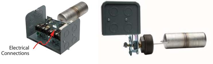
For **Duplex Condensate Return Pumps** the Float Switch is replaced with a Mechanical Alternator. The Mechanical Alternator is attached to a float and activates only one pump at a time in an alternating manner. The Mechanical Alternator switches power between the two motors so that the runtime of each pump is shared, allowing the system to continue operation in the event of a single pump failure.
