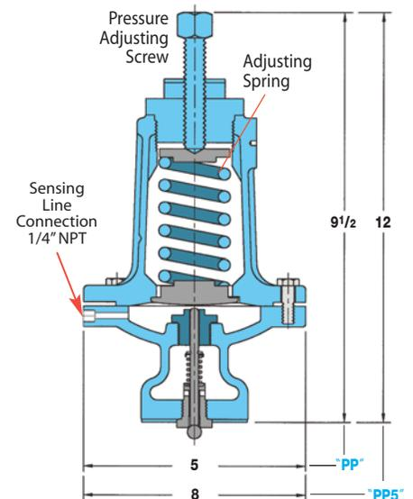
Pressure Regulating with PP & PP5 Spring-loaded Pilot
