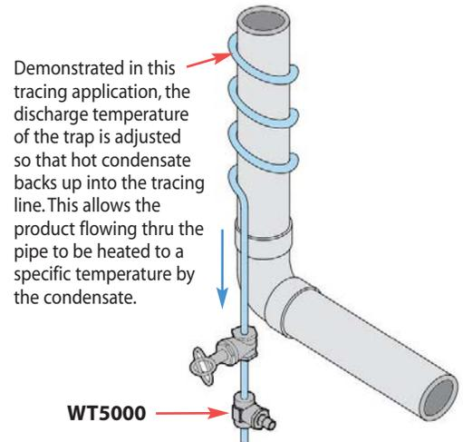
**T = Initial Opening Temperature of the Trap** can be set from 120°F to 390°F
