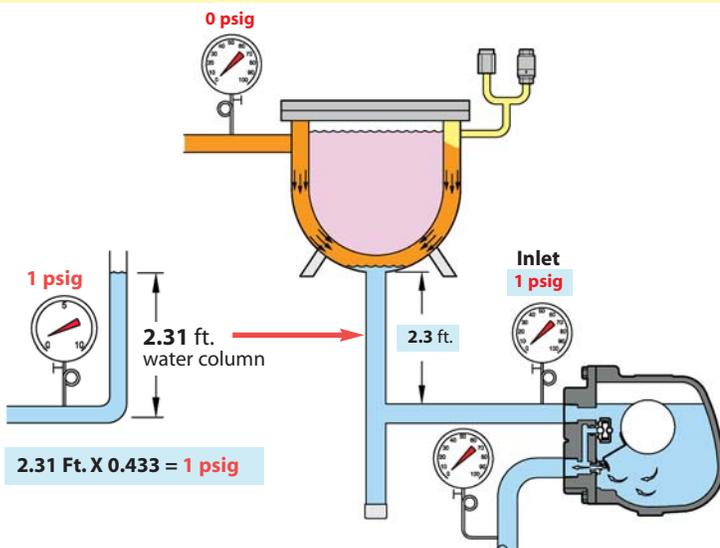
When set temperature of the process fluid is reached, the steam pressure inside the jacketed kettle may reduce to 0 PSIG or even go into Vacuum. To promote condensate drainage, the steam trap is placed a certain distance below the process equipment.
