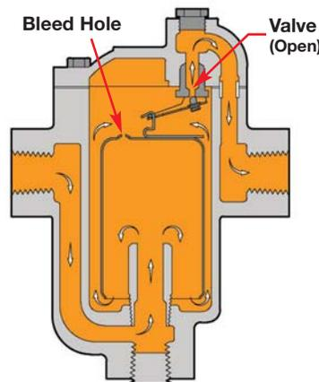
**D) Potential Failure Mode:** Bucket traps must maintain a water prime to function properly. If the prime is lost, the bucket will remain in the down position with the valve open, and live steam will be discharged from the system.
