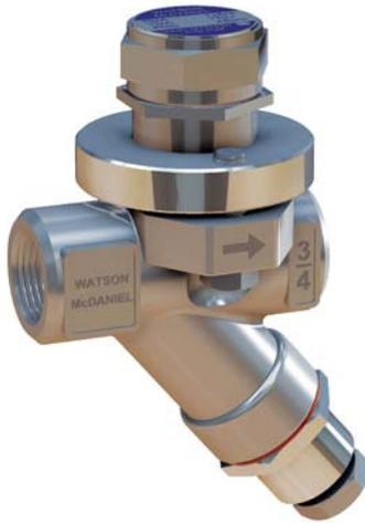
UTD450 Trap Module should be oriented with cap facing Upwards. Therefore it should only be used with Horizontal Piping, as shown.
