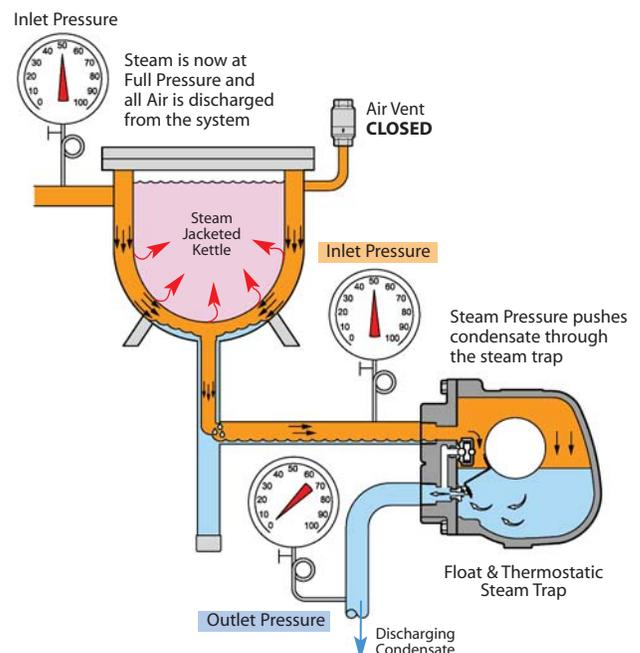
**Typical Ways Steam Traps are Installed ... and how this affects the differential pressure.**
