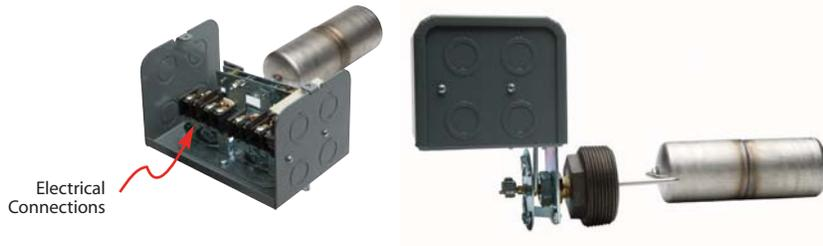
On Duplex units, the standard float switch is replaced with a Mechanical Alternator float switch to alternate operation between the two pumps. Must be ordered separately. An Electric Alternator is also an option.
