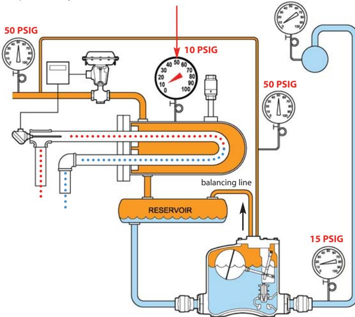
**Vent Outlet:** Open position, allowing pressure in the pump tank to equal pressure in the heat exchanger, allowing condensate to freely enter Pump-Trap by gravity.
