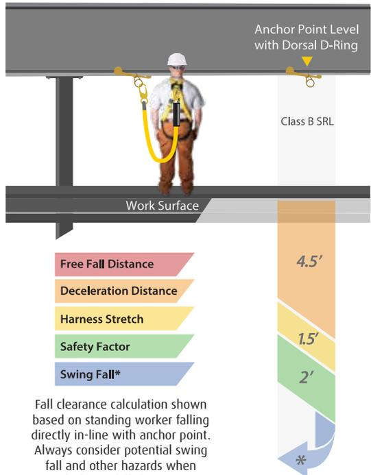
**Compatibility:** When making connections with Halo Web SRL, eliminate all possibility of roll-out. Roll-out occurs when interference between a hook and the attachment point causes the hook gate to unintentionally open and release. All connections must be selected and deemed compatible with Halo Web SRL by a Competent Person. All connector gates must be self-closing and self-locking, and withstand minimum loads of 3,600 lbs. See the following for examples of compatible/incompatible connections:
