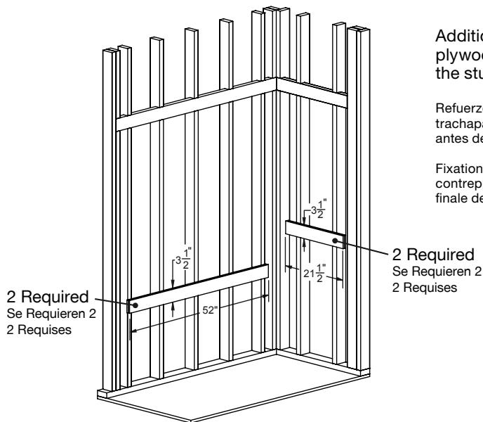
Additional bracing is required before grab bars are installed. Using  $\frac{1}{2}$ " plywood, reference the suggested measurements and attach bracing to the studs before final installation of the bathtub wall unit.
