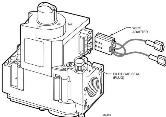
Fig. 10—VR8345 wiring connections in direct spark ignition system (single rod application).
