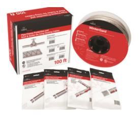
nVent RAYCHEM WinterGard self-regulating trace heating cables provide energy efficient and easy to use solutions for pipe freeze protection. This TruckPak kit includes heating cable, two H900 hardwired power/end seal kits, one H910 splice/tee kit, and one H903 application tape. Available as 120 V, 100 ft, 3W/ft or 6W/ft.
