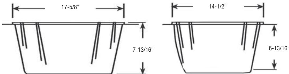
Note: All dimensions and specifications are nominal and may vary: Dimensions of 8" and greater have a tolerance of +3%. Dimensions less than 8" have a tolerance of +5%. Please utilize the current cutout template for countertop cutouts.
