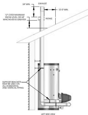
SIDEWALL VENTING WITH CONCENTRIC VENT KIT
