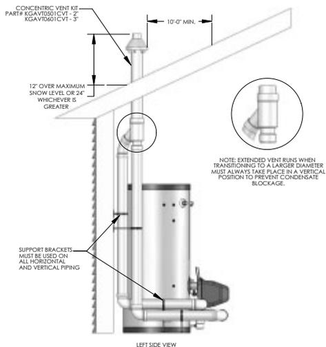
**NOTE: When placing support brackets on vent piping, the first bracket must be within 1 foot of the appliance and the balance at 4 foot intervals on the vent pipe.**
