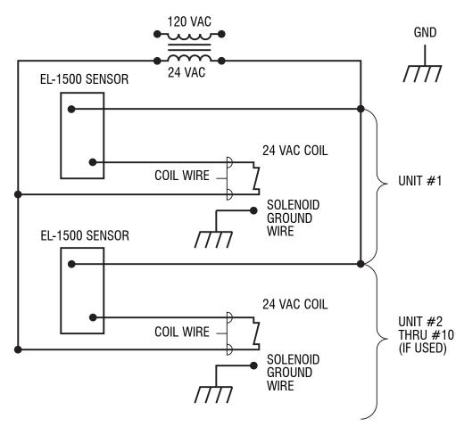
**IMPORTANT:** Early Models of the Sensor were made with four (4) Wire Leads. When replacing a four (4) Wire EL-150 Sensor with a three (3) Wire EL-150 Sensor the Black Lead replaces the Blue Lead, the Red Lead replaces the Yellow Lead and the White Lead combines and replaces the Brown & Red Leads.
