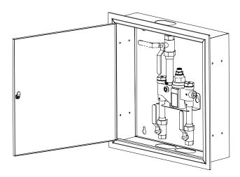
Inlet Connections: 3/4" NPT Outlet Connection: 1" NPT Temperature Range: 85–135°F Maximum Pressure: 125 PSIG Inlet Temperature Hot: 120–180°F Inlet Temperature Cold: 39–80°F Minimum Temperature Differential (between hot supply & valve set point): 20°F
