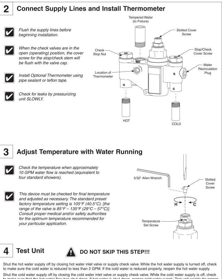
Shut the cold water supply off by closing the cold water inlet valve or supply check valve. While the cold water supply is off, check to make sure that the hot water flow has shut down. If hot water is shut down, reopen cold water supply. Test unit weekly for proper function and desired set temperature.
