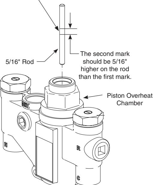
**D** Push the mechanism up and down several times to make sure the piston moves smoothly and consistently. If it is not consistent, repeat Procedure C until it moves freely, or replace. Contact your Bradley representative and ask for Piston/Liner Kit (part number S65-184).
