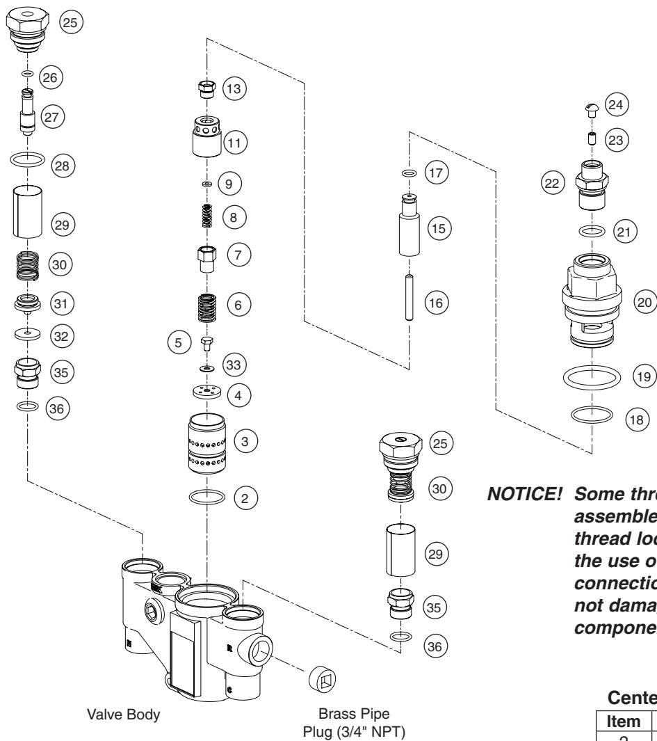
**NOTICE!** Some threaded joints are assembled using high strength thread lock and may require the use of heat to loosen the connection. Use caution to not damage O-rings or other components.
