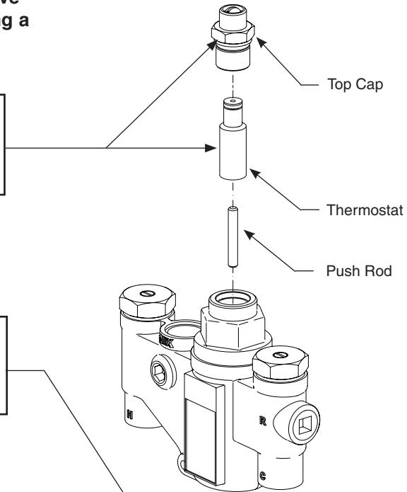
**B** Insert a 5/16" dia. rod into the valve and into the piston overheat chamber. Mark the length of the rod inside the valve. Push the rod until the piston stops and mark the new length.
