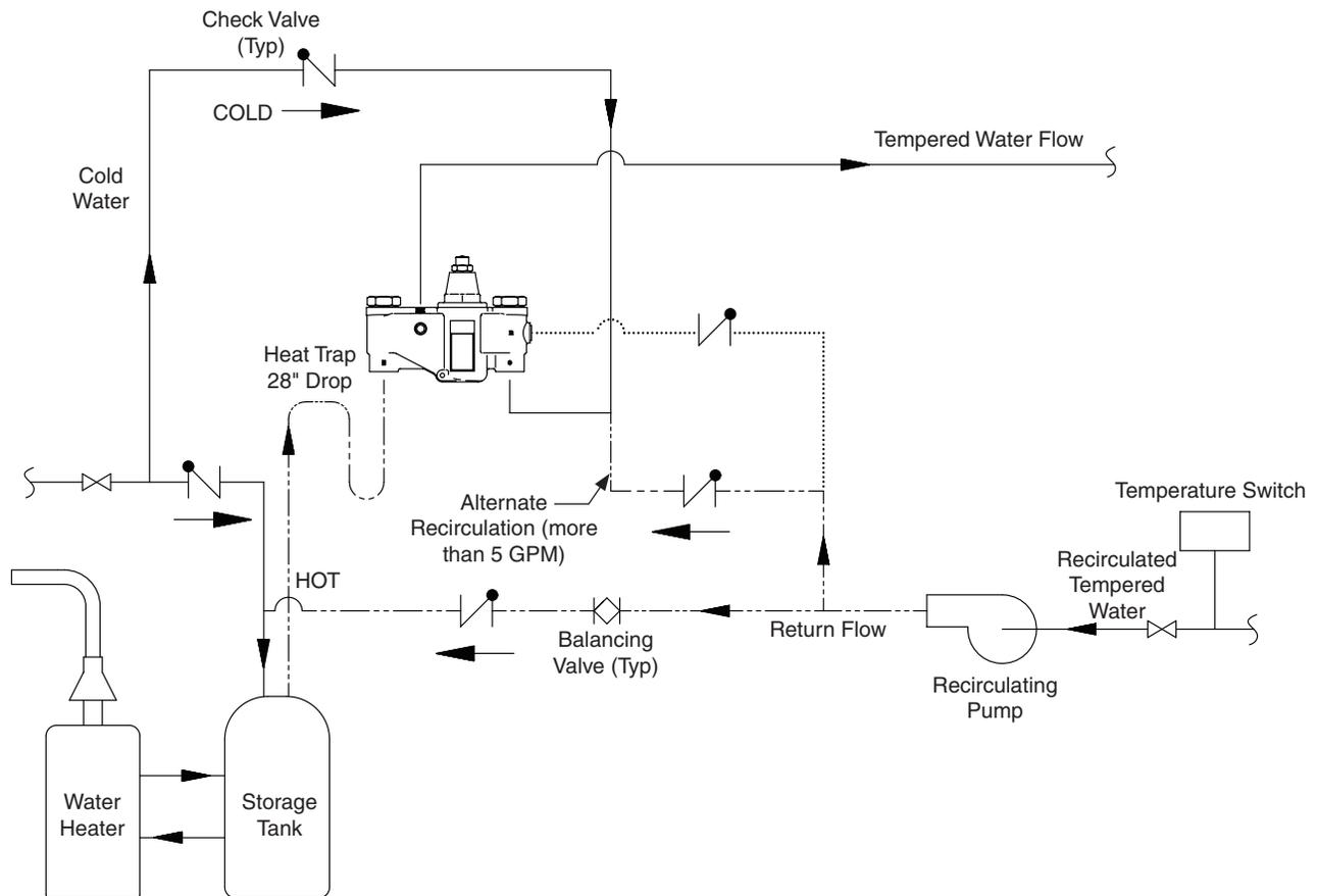
1. Turn off the recirculating pump and turn on the water supply (a water flow rate of 10-15 GPM is required).
