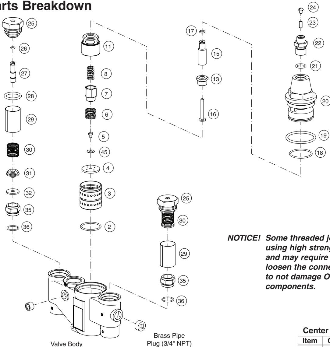
**NOTICE!** Some threaded joints are assembled using high strength thread lock and may require the use of heat to loosen the connection. Use caution to not damage O-rings or other components.
