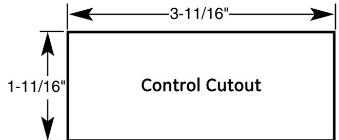
We recommend that the cutout in granite or other hard surfaces be made before the countertop is installed.
