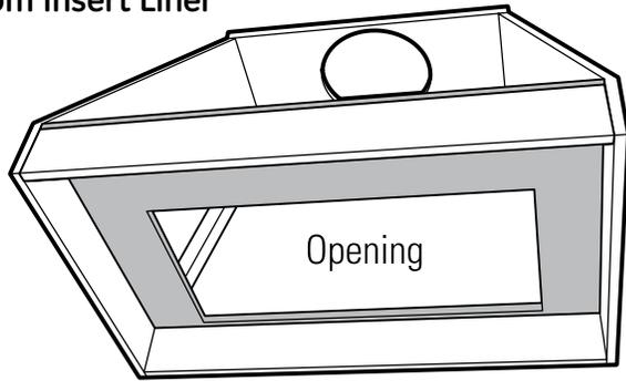
The custom canopy must be sized to fit the insert sleeve. Construct the canopy with an opening that is: 38-3/4"W x 13-3/16"D. The opening must be constructed of 3/4" thick material to allow the sleeve locking clips to engage.
