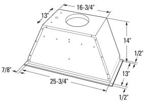
The bottom edge of the insert sleeve has a 7/8" wide flange on the sides and a 1/2" wide flange on the front and back.
