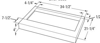
A stainless steel liner is shipped with each hood insert. This non-combustible liner protects the underside of the canopy.
