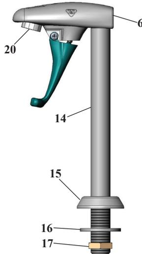
4. Apply teflon tape or pipe joint compound to threads of no.14, connect to water supply line inlet.
