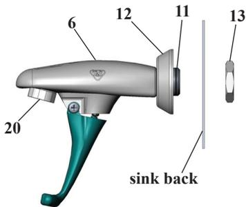
2. Drill 7/8" hole in sheet metal. Insert no.6 through hole and screw no.13 on back of no.6, leaving no.12 free to turn.
