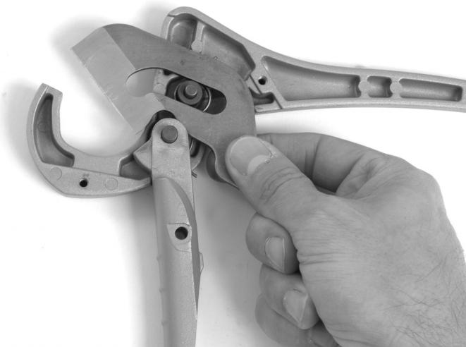
Figure 2 – Blade Removal
