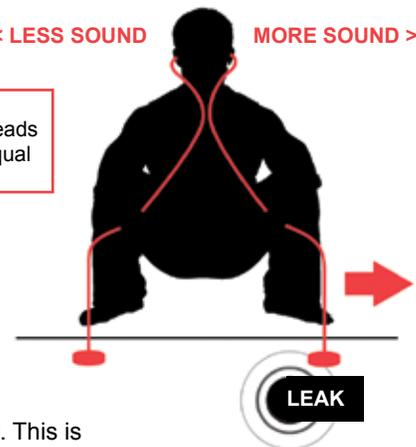
**NOTE 1:** The instrument works best when it is free standing, since the circulation of blood in the hands will set up detectable vibrations.
