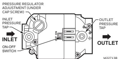
Fig. 2. Top view of VR8205S, T combination gas control.
