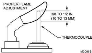
Fig. 6. Proper flame adjustment.
