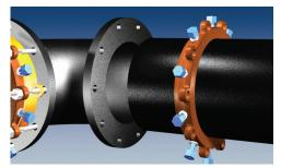
2. Cut the pipe to the required length. Clean the end of the pipe for a length approximately one foot using a wire brush if needed, removing all excess paint and foreign material. Also clean the opposing flange to be connected to the 2100. Place the 2100 restraint ring on the clean pipe with the lip facing the plain end.
