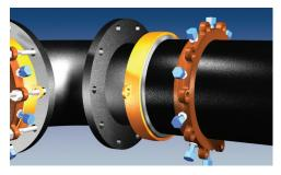
4. Place the O-ring into the groove of the 2100 Gasket Ring. (This step may have been completed at the factory, check Gasket Ring to see if O-ring is already in place.) Place the Gasket Ring on the pipe with the O-ring facing the pipe end and the gasket recess facing the EBAA-Seal (or transition) Gasket and restraint ring.
