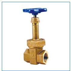
**Specifications UPC** Code 039923620224 Gate Valve Type Valve Size **Connection Type** T -- Female NPT Thread (FIPT) **Seat Material** Bronze Material Bronze **Description** T174A 1 THD 300# RS GATE BRZ Standard Handwheel **Valve Operator** Multi-Turn **Turns/Operation** 3.370 lb Weight
