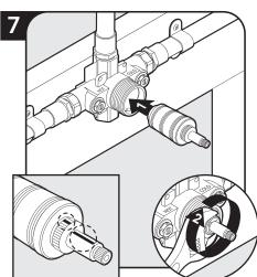
**Note:** Make sure black alignment marks on cartridge line up with marks on stem and are on top of the cartridge.
