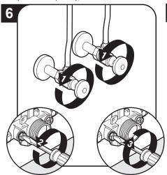
Turn on water supply and open integral stops to flush lines. Turn off integral stops.
