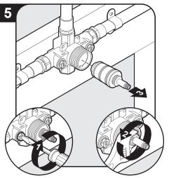
Close integral stops and remove cartridge.
