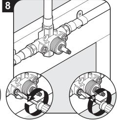
Open integral stops to flush lines to volume control. Turn off integral stops. Replace Plaster tile guide B.
