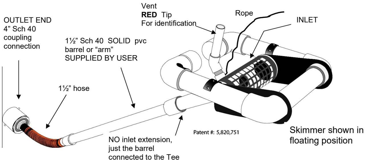
2. Glue the 1½" Sch 40 **barrel** pipe to the 1½" white coupling on the **hose**.
