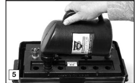
The hole is marked with an arrow. Replace the battery cables...the WHITE wire to the NEGATIVE (-) post, and the BLACK wire to the POSITIVE (+) post. Replace the wing nuts and tighten.
